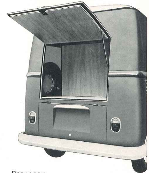
Rear door: width 35.4 inches, height 28.7 inches
