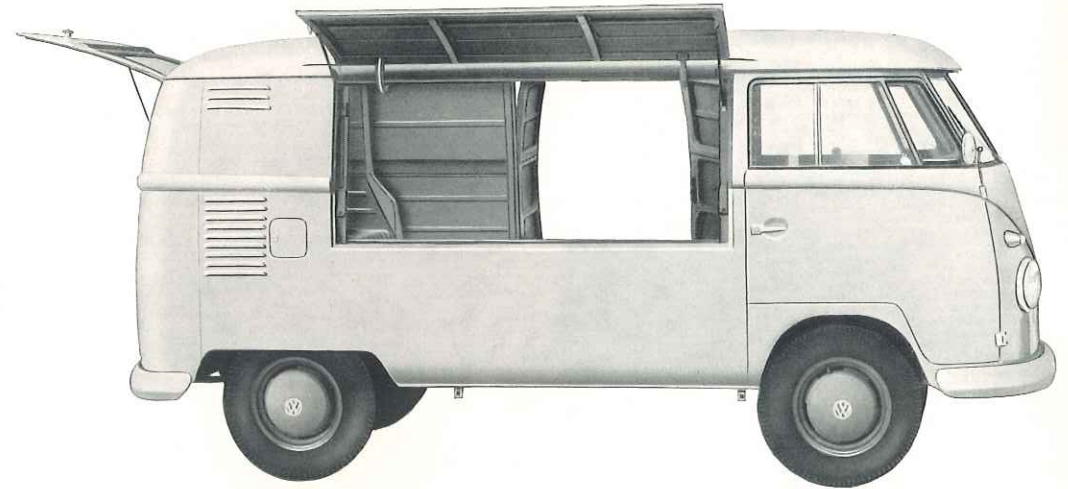
The VW Mobile Shop in standard roof version Sales flap: height 26 inches, width 64.8 inches Height from ground to lower edge of sales flap: approx. 33.4 inches
