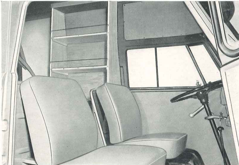
Driver's cab with divided front seat and access to sales room
