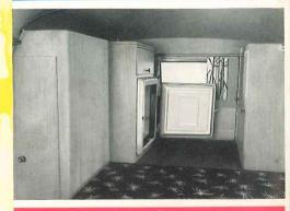
The furnishings also include a wardrobe and a cupboard with compartments for chothing, crockery etc. which is fitted directly above the refrigerator. (Absorber, capacity 40 ltrs. functions efficiently even in fierce heat.)
