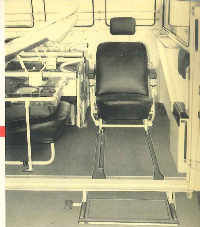
The carrying chair is extremely comfortable and convenient — the back can be adjusted to various angles.
