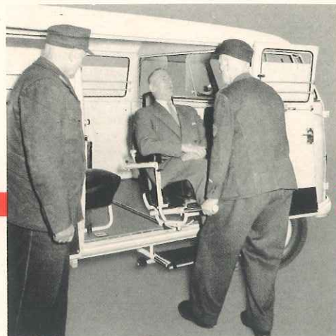
Without moving the patient, the carrying chair is slid in on rails.
